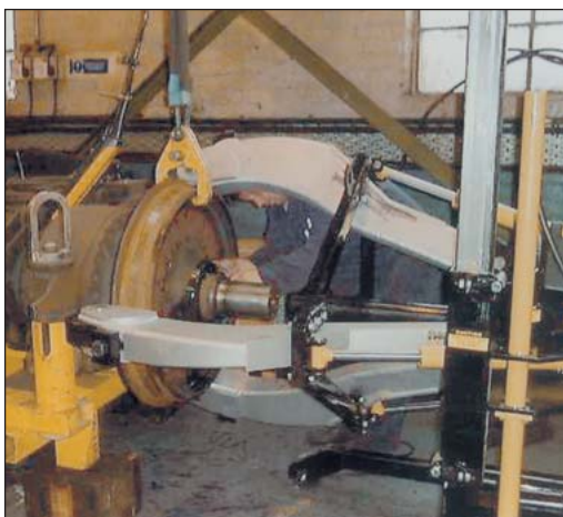
◀ The EPH-1003 quickly and easily removes this drive sheave from its shaft.
